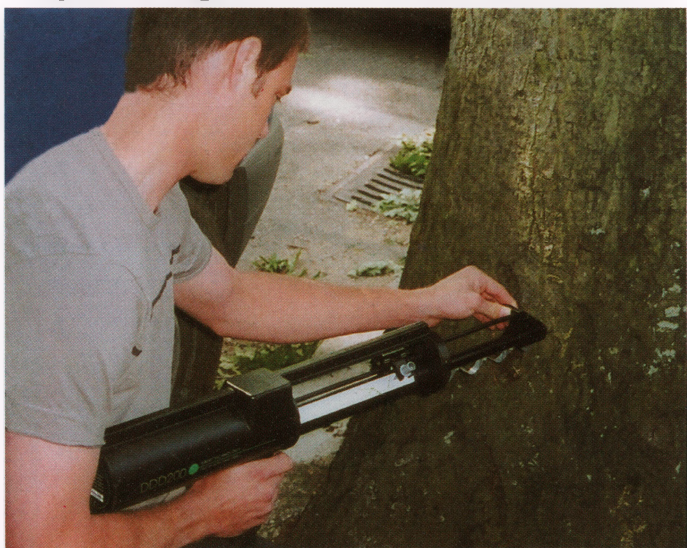
Tree Officer Fred Micoud demonstrates the Decay Detection Drill to residents.
